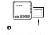
After the wiring of switch module is done, long press the reset key for about 5 seconds until the indicator light ash quickly for pairing mode(If you wait more than 180 seconds you need to repeat this passage). If it's not the correct item, pls long press for about 10 seconds until the indicator light flash quickly to change it to another item.
