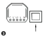
After the wiring of switch module is done, press the traditional switch to turn ON/OFF cycle for 5 times (keep time interval not too short) until the indicator light flash quickly for pairing mode.
