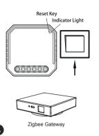
After the wiring of switch module is done, press the reset key for about 10 seconds or turn on/off the traditional curtain for 5 times until the indicator light inside the module is flashing quickly for pairing.
