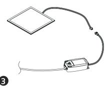
Switch the on/off button for 5 times until the light connected to the driver is flashing, then the light connected to the driver ready for pairing.
